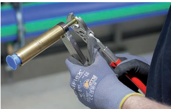
5. Remove the drilling residues from the core bit using a special tool.
