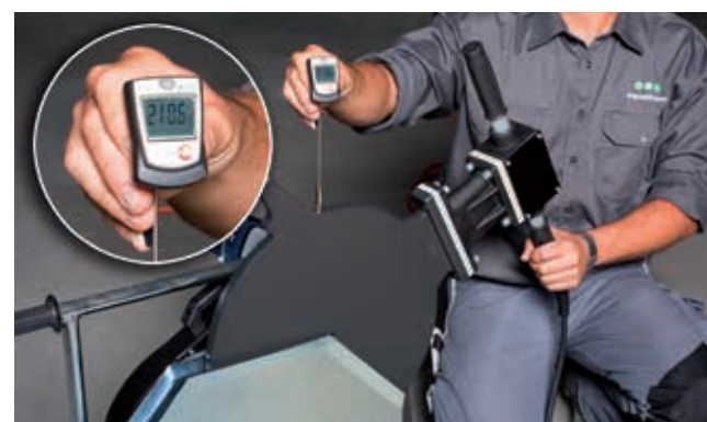
Temperature measurement on aquatherm butt fusion machine
