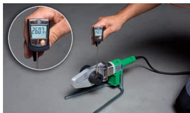
Temperature measurement on the aquatherm hand welder (800 W)
