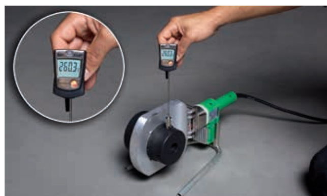
Temperature measurement on the aquatherm hand welder (1400 W)
