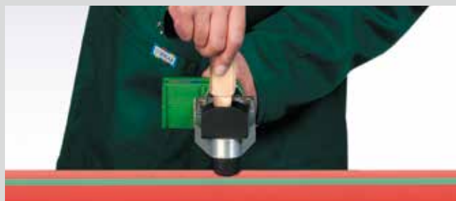
Heat-up of pipe...
