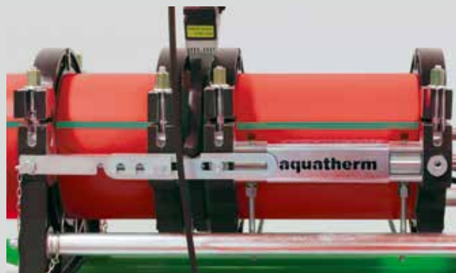
Positioning of heating element
