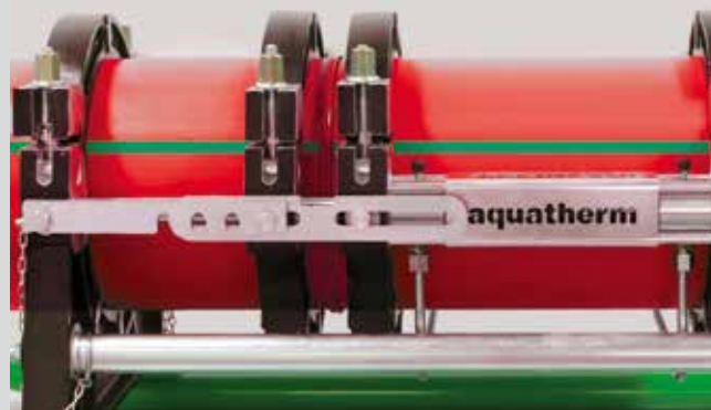
Join the pipes, cool down under pressure
