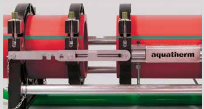
The parts to be welded are fixed and aligned respectively, the milling machine is used
