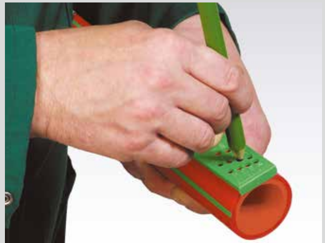
Marking of the welding depth
