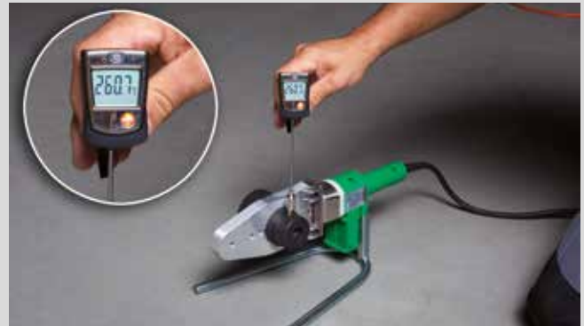
Measurement of temperature at the aquatherm manual welding device (800W)
