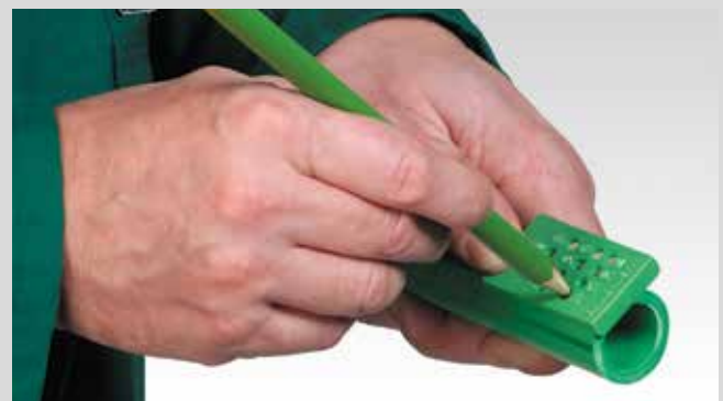
Marking of the welding depth
